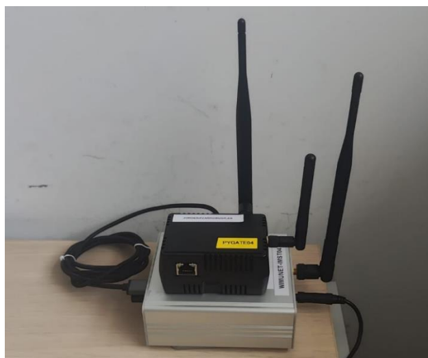
Figure 3. Pair IMST Lite and Pycom Pygate gateways (example of gateways located at CSIC-UGR).
